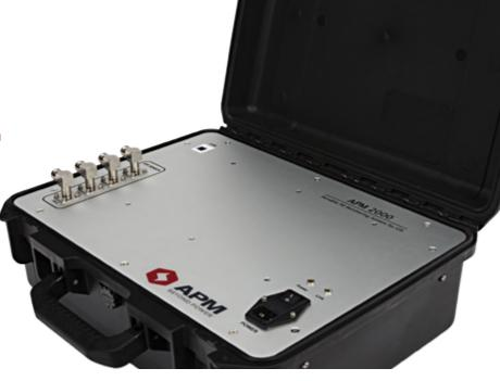
APM 2000 detects and alerts various defects inside EHV/MV equipment by analyzing UHF signals generated by partial discharge. It monitors, records and analyzes PD signal continuously and alerts the condition of EHV/MV equipment with light-weight and small-sized equipment.
